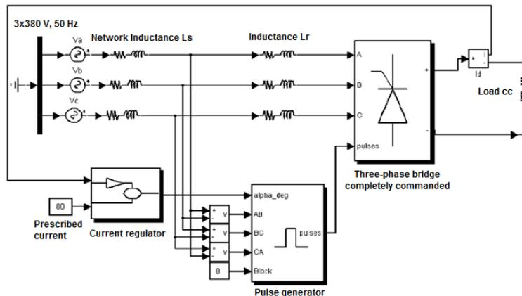
**Fig. 3.** Simulink model of three-phase rectifier with thyristors
