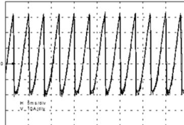
**Fig. 9.** The reference signal and the measured value of the filter current on the q axis.
