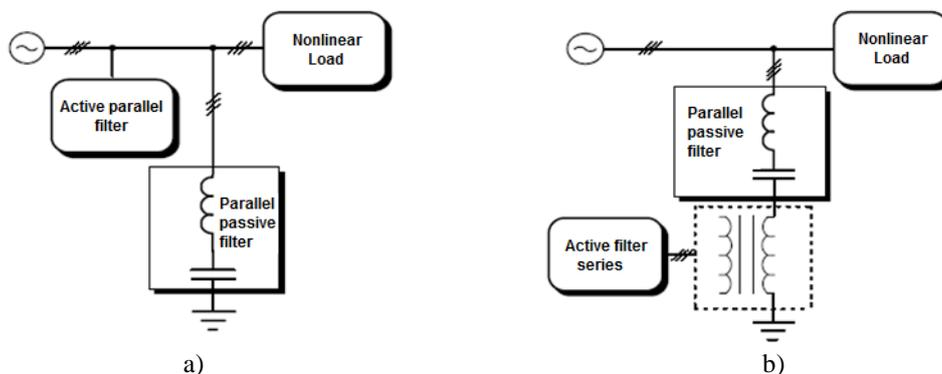
**Fig.2.** Combinations of filters a) Active parallel filter – parallel passive filter;
